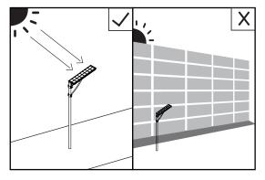
When install the integrated solar street light, please choose a position with enough sunshine and fully exposure. Please note the solar panel must be fully exposure, without any shelter.
