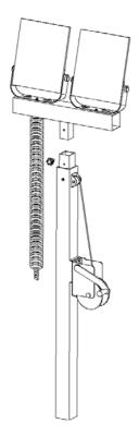
Step 2: Insert the upper lamp head with the lamp into the inner lamp pole, and twist the M8 hand screw nut.
