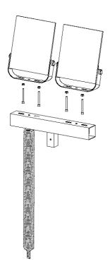
Step 1: Fix the LED lamp holder on the upper lamp holder with screws and nuts, and connect the wires.
