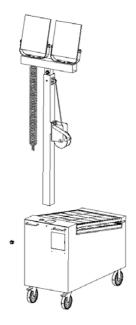
Step 3: Insert the light pole with the lamp, and tighten the M8 hand-twisted nut that fixes the square cabinet and the light pole.
