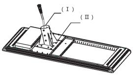
4. Drill a 10\*0.70" through hole at 5.19" from the top of the pole to fix the bracket (Can use the bracket to locate the hole position).
