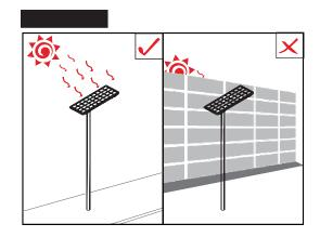
When install the integrated solar street light, please choose a position with enough sunshine and fully exposed. Please note the solar panel must be fully exposed, without any shelter.
