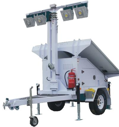
The SP-SL600-4 is a solar powered LED light tower that provides a safe and effective way for operators to quickly deploy high powered lights. This light allows for easy transportation and easy setup. Unlike other types of lamps, this one has LED light. These types of lights have a much longer lifetime than a normal bulb. Our portable, solar powered light trailer helps you to reduce your energy consumption, and it will illuminate large areas at great distances.
