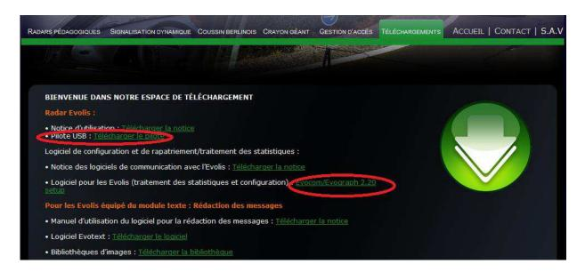
Download the USB driver. Run the setup to start the installation. A black window that shows the progress of the installation will appear.
