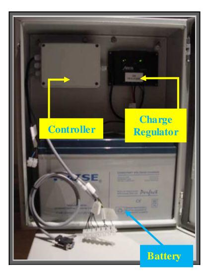
Place the battery inside of the box using caution due to its weight. It should look like the above picture. In the box you will have one charge regulator, one controller, the battery and several cables. Next, you must connect the 2 wires of the charge regulator to the battery. Connect the red wire to the positive terminal (+) and the black wire to the negative terminal (-). Now you should see 2 Green or yellow LEDs illuminate.
