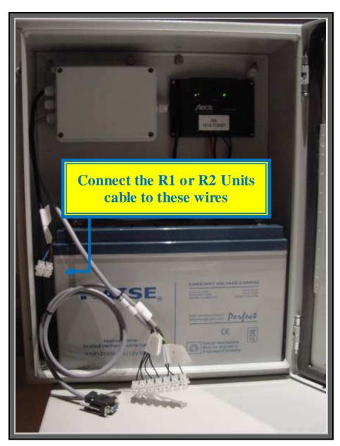
Now you can connect the road studs cable into the output controller cable for the R1 or R2. Connect the blue wire of one cable with the other and the same for the brown wire
